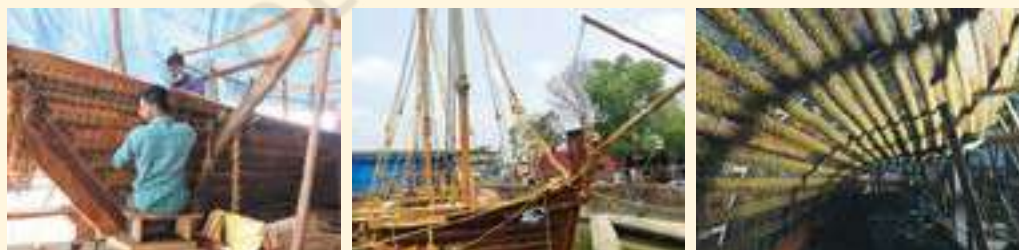
Fig. 7.9. Re-creation of a 5th-century stitched ship
