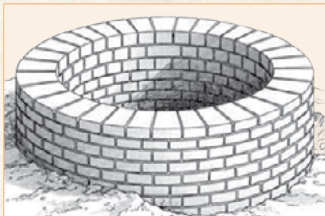
Fig. 3.14. A simplified sketch of a typical Harappan well built with trapezoid-shaped bricks.
